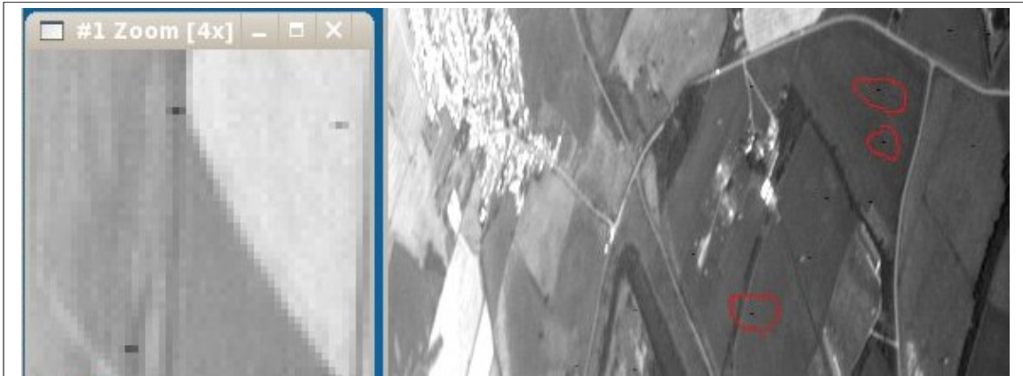
Figure 5a: band 2 of ATM showing suspected electrical interference (dark speckles)
