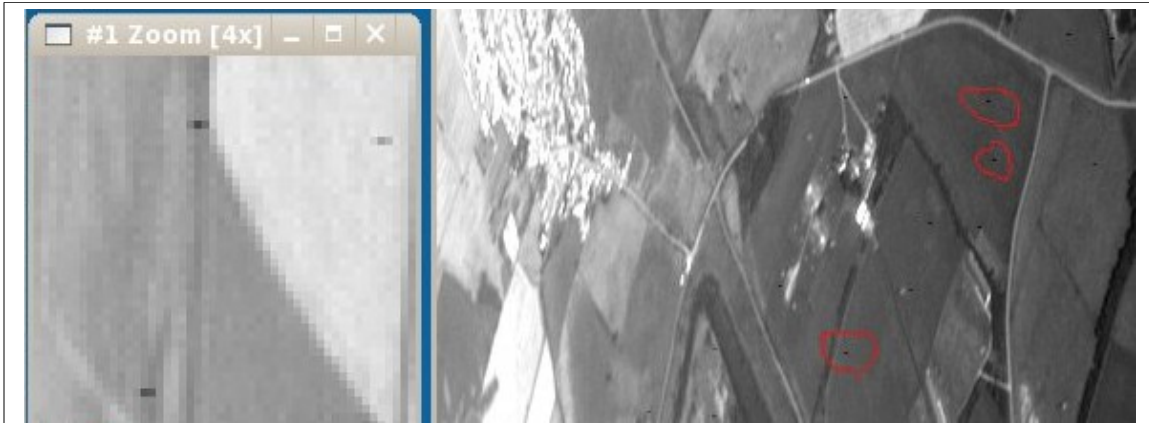
Figure 6a: band 2 of ATM showing suspected electrical interference (dark speckles)
