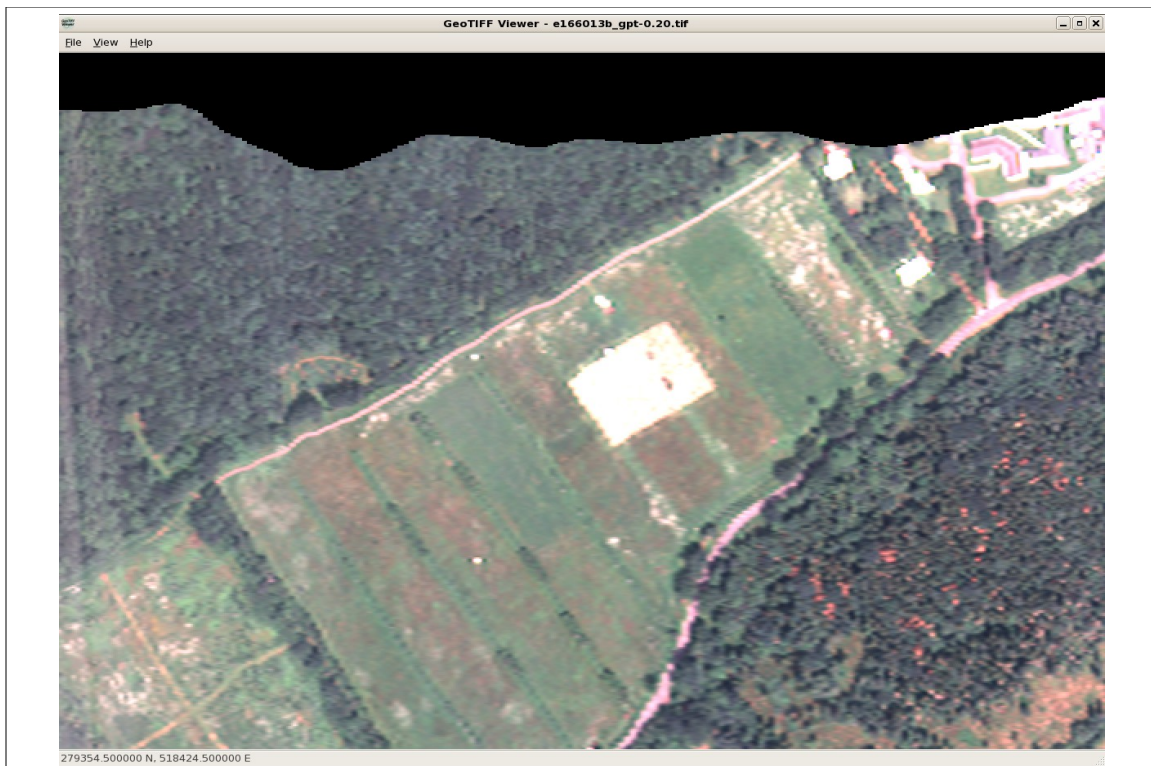
Figure 1a: timing error in an Eagle line
