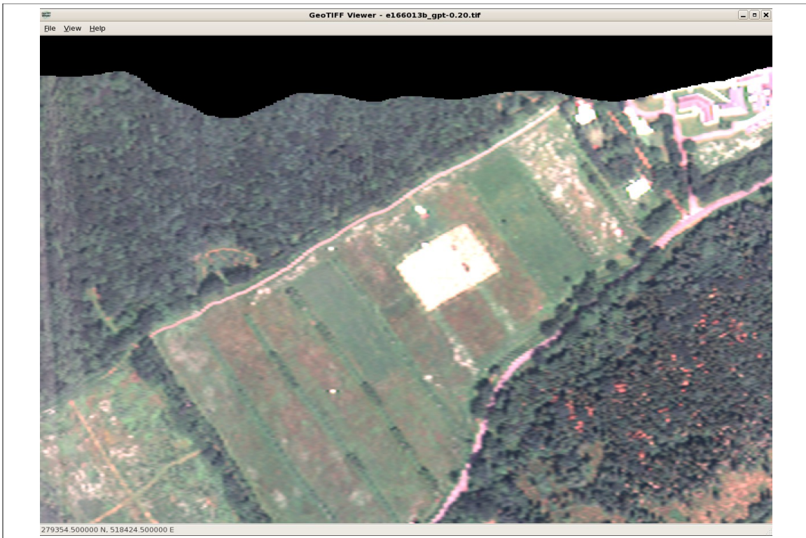
Figure 1a: timing error in an Eagle line
