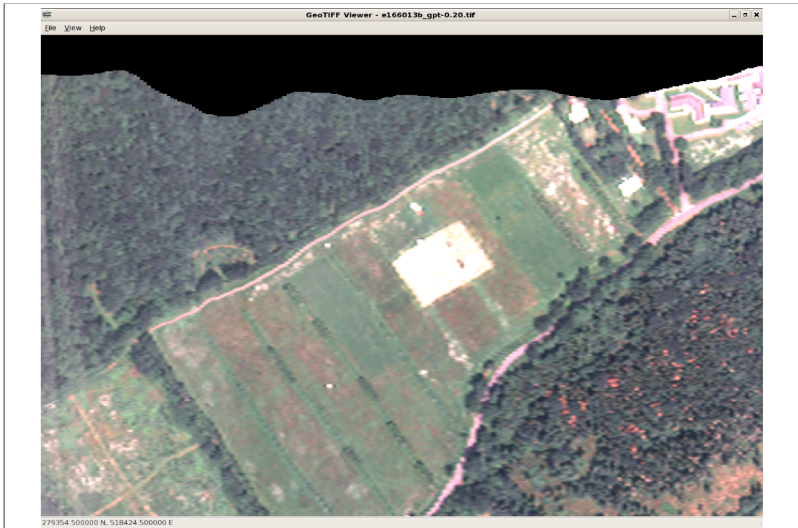
Figure 1a: timing error in an Eagle line
