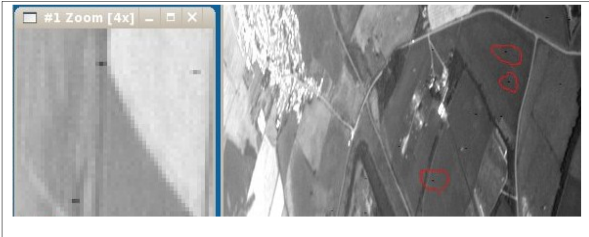
Figure 3a: band 2 of ATM showing suspected electrical interference (dark speckles)
