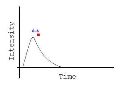
Figure 2: Waveform peak and corresponding discrete return (red square) occur at different times.
