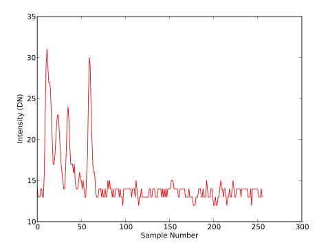
Figure 1: Example Waveform for a forested area.
