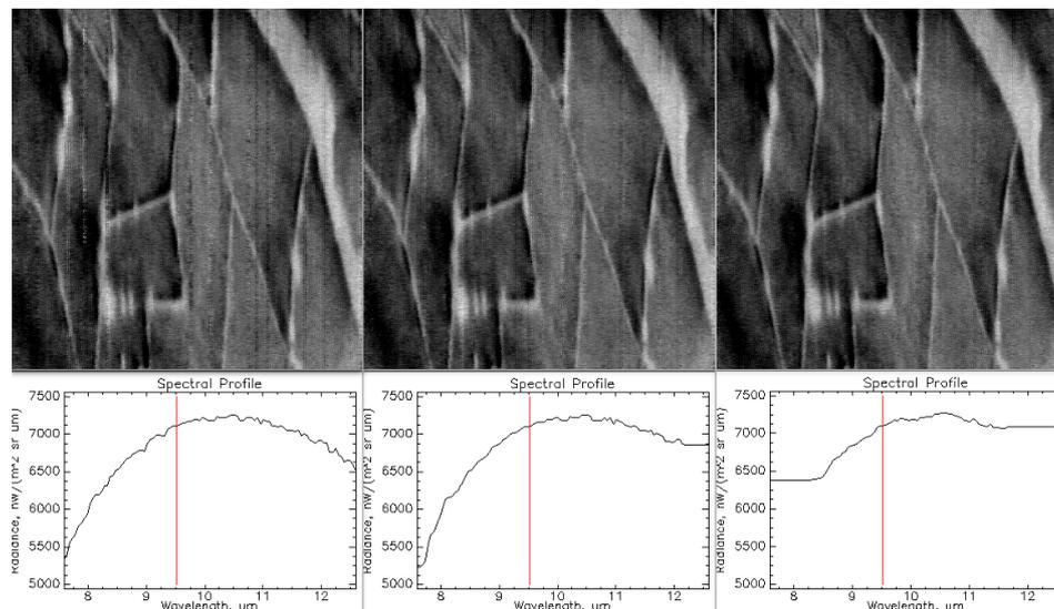
Figure 5: *Example image processed with decreasing blinker threshold. The red vertical lines on the spectra indicate the band displayed in the images above.*
