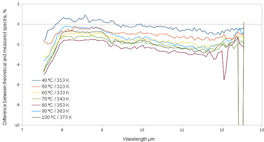
Figure 4: *Percentage spectral error at different target temperatures. Some of the error may be due to inaccuracy in the target black body temperature.*
